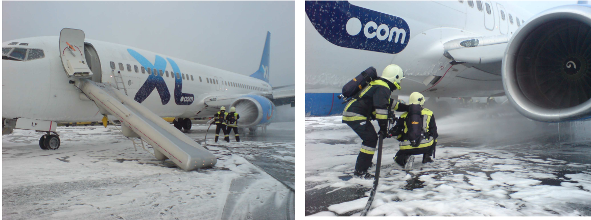
Slides 5 and 6: Cooling of the engine and the landing gear
