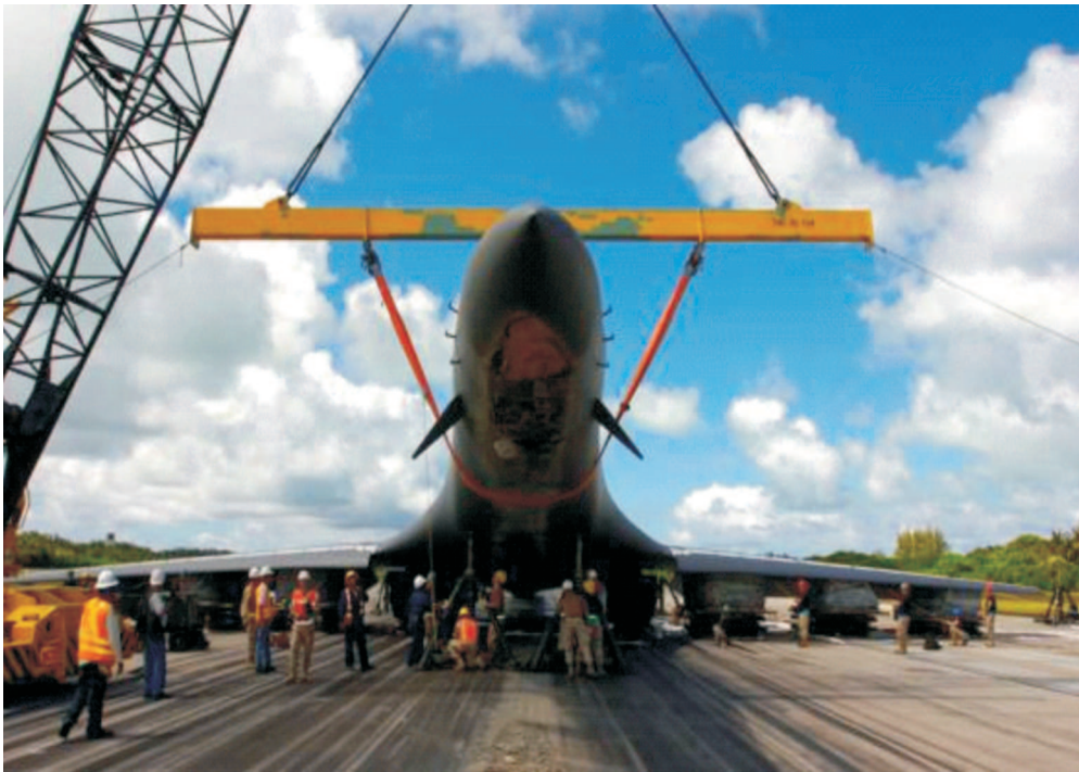
Fig. 3. Special removal equipment [5]
